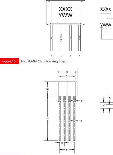
Figure.17 Flat TO-94 Package Drawing
